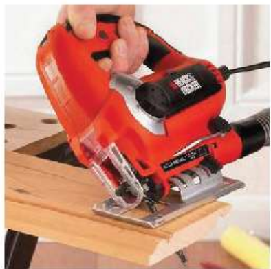
38-rasm. Elektr lobzik kesish burchagining og'ishi
