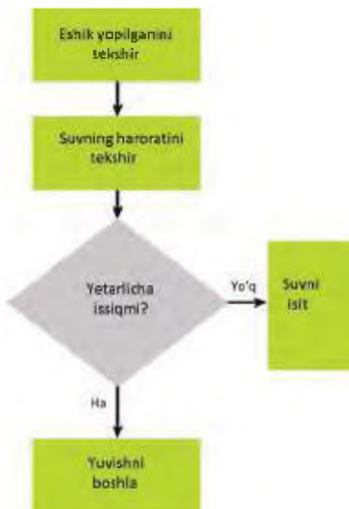
2.06-rasm. Kir yuvish mashinasida harorat sensorining qo'llanishi.
